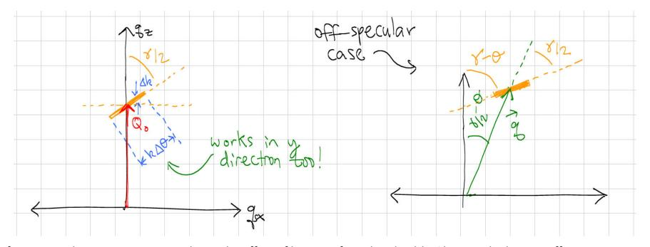
Before proceeding it is easy to see what is the effect of having a finite bandwidth,  $\Delta k$ . Here the biggest effect is on q itself. In this geometry, in sample coordinates,  $q = (0,0,2 \ k \sin \theta)$ . So a finite bandwidth just smears our line segment in the (longitudinal) z direction, making a trapezoid as shown.
